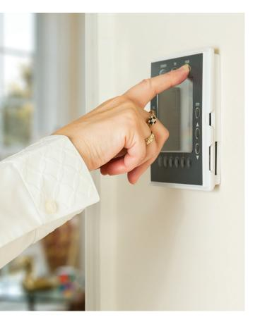
Modern heat pumps are designed to automatically adjust to changing conditions, so they work best when the temperature settings are left alone. **Once you've found your comfort number, leave it be.** Modern heat pumps use less energy when they maintain the temperature.
